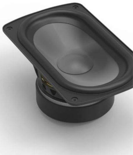
△ THE RACE-TRACK SHAPE OF THE BASS DRIVERS ALLOWS GOLDENEAR TO MAXIMISE THE CONE AREA ON THE FRONT BAFFLE WHILST AT THE SAME TIME MINIMISING THE WIDTH OF THAT BAFFLE, WHICH HAS THE EFFECT OF IMPROVING BOTH DISPERSION AND IMAGING.
