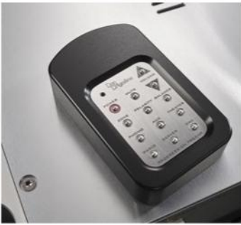
△ THE REMOTE CONTROL IS NOT YOUR 'STANDARD' DEVICE NOT ONLY BECAUSE OF ITS DESIGN AND SHAPE, BUT ALSO BECAUSE IT TRANSMITS CONTROL SIGNALS VIA BLUETOOTH, NOT INFRARED.
