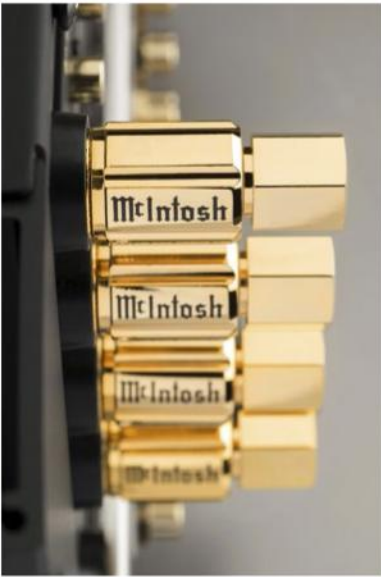
△ THE SPEAKER TERMINALS ARE UNUSUAL BECAUSE EVEN THOUGH THE MA9000 CAN DRIVE ONLY A SINGLE PAIR OF SPEAKERS, THERE ARE EIGHT BINDING POSTS: FOUR EACH AT EITHER END OF THE REAR PANEL.
